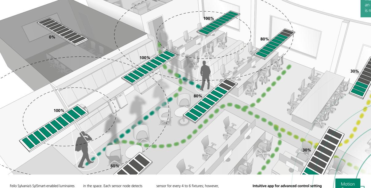
feature a Sensor Node that is integrated into each luminaire during manufacture. Each Sensor Node contains a motion sensor, communications module, ambient light sensor and an intelligent microprocessor. As soon as a luminaire is connected to the power supply, it will start detecting.
